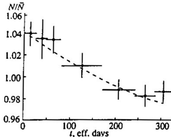
Figure 2 – The evolving antineutrino rate  $N$ , versus time in days, relative to  $\bar{N}$ , the mean value of the rate, as measured in an experiment at Rovno<sup>5</sup>. The gradual drop in the relative rate, arising from the increasing fraction of plutonium in the core as the reactor proceeds through its fuel consumption cycle, is clearly seen in the data (points with error bars) and confirmed by a model of the reactor core (dashed line).
