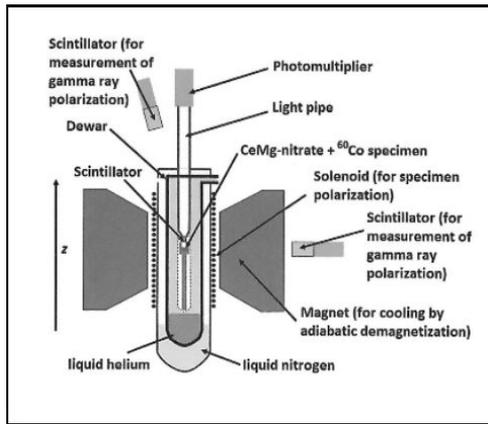
Figure 1 – Parity Experimental Arrangement.
