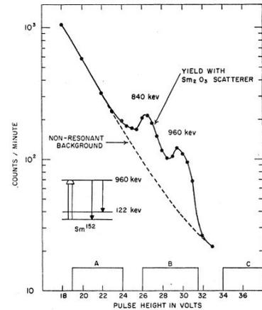
Figure 7 – Resonant scattering energy spectrum.
