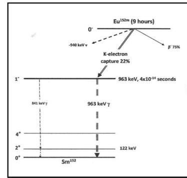
Figure 5 – Helicity experiment decay scheme.
