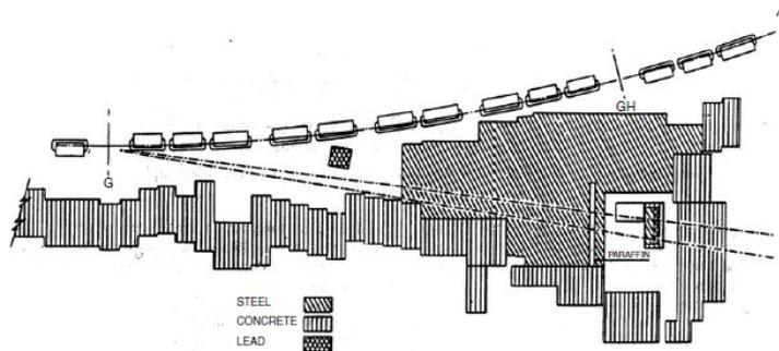
Figure 12 – Neutrinos Beam, Target and Shielding.
