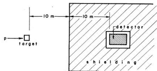
Figure 10 – Experimental arrangement for a neutrino beam
