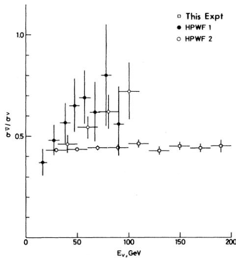
Figure 6 – Ratio between antineutrino and neutrino total cross-sections as a function of neutrino energy from CDHS (open squares) and HPWF (circles) experiments.
