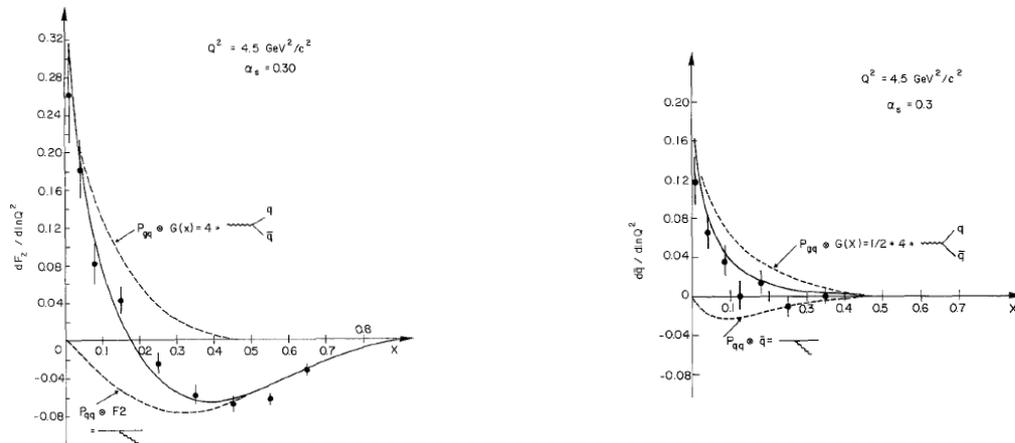
Figure 10 – Left: Slope of structure function  $dF_2/d\ln Q^2$  versus  $x$  and contributions from gluon bremsstrahlung and gluon pair production. Right: Slope of structure function  $d\bar{q}/d\ln Q^2$  versus  $x$ . From ref. <sup>13</sup>.
