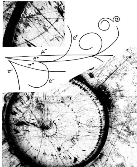
Figure 3 – Observation of charm production and decay in the 15-ft bubble chamber at Fermilab<sup>4</sup>.
