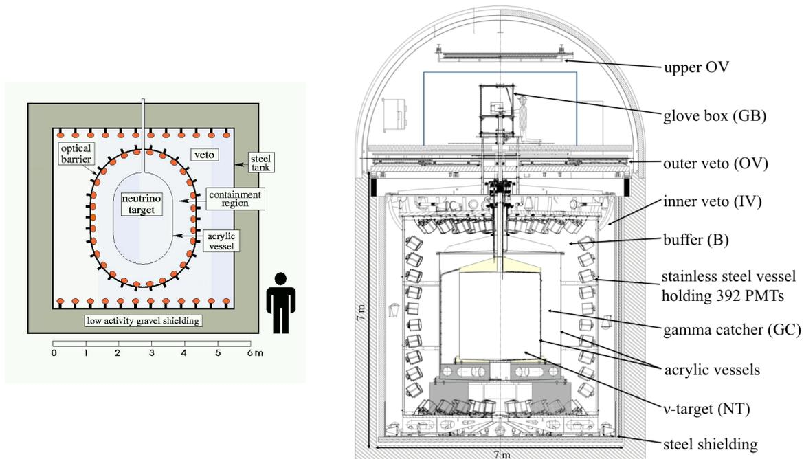
Figure 4 – (Left): Sketch of the Chooz detector. (Right): Sketch of the Double Chooz detector, a novel 4-large-volume detector design proposed by the Double Chooz collaboration and adopted by the RENO and Daya Bay experiments.
