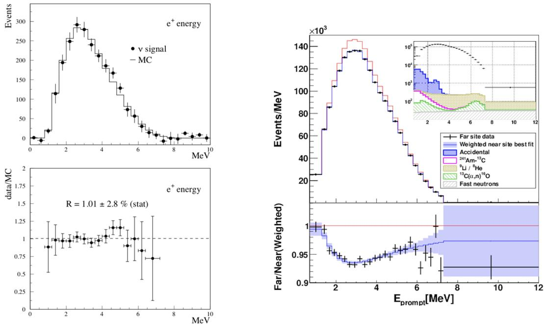
Figure 6 – (Left): The Chooz positron spectrum; the bottom panel shows the ratios of data over predictions with no oscillation. (Right): The Daya Bay background-subtracted spectrum at the far site (black points) and the expectation derived from near-site measurements excluding (red line) or including (blue line) the best-fit oscillation; the bottom panel shows the ratios of data over predictions with no oscillation<sup>30</sup>.
