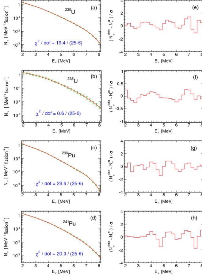
Figure 1 – Reactor antineutrino spectra as reevaluated in 2011 by the Saclay group<sup>2,3</sup>.
