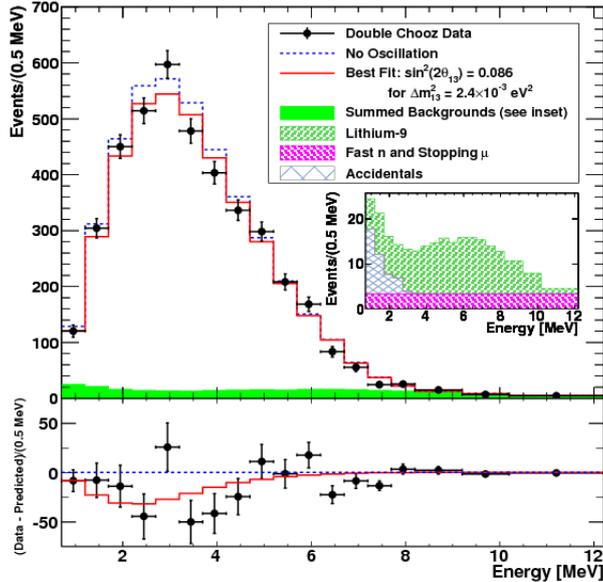
Figure 5 – First results of the Double Chooz experiment in 2011, providing the first evidence for a non-zero value of the  $\theta_{13}$  mixing angle<sup>27</sup>.
