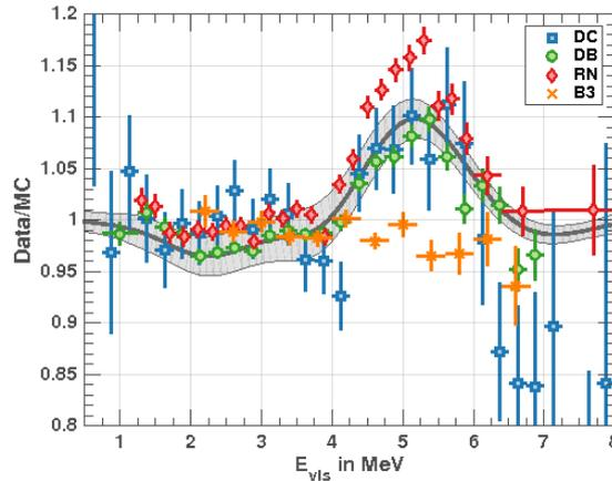
Figure 8 – Ratio of observed reactor antineutrino spectra to current best predictions<sup>2,3</sup>. Despite similar fuel compositions, Double Chooz (DC), Daya Bay (DB) and RENO (RN) display significant deviations around 5 MeV, while Bugey 3 (B3) does not. Figure taken from ref.<sup>36</sup>.
