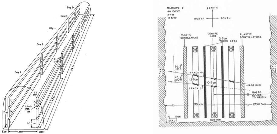
Figure 3 – The left panel is a scheme of the CWI detector [taken from<sup>98</sup>]. The right panel shows one intriguing event detected by the KGF detector with two up-going tracks that originate from the same point (in the rock (or in the air near the rock) to the right of the figure) [taken from<sup>92</sup>].
