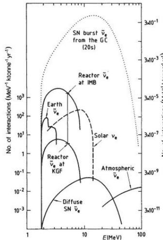
Figure 2 – Number of events expected for different antineutrino and neutrino sources (reactors, supernovae, Sun, atmospheric) between 1 and 100 MeV <sup>2</sup>.
